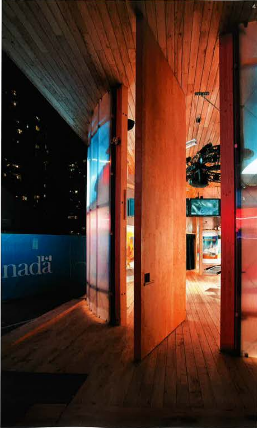
SPACED BOARDS ON THE FLOOR AND CEILING, TOGETHER WITH AN OVERSIZED PIVOTING DOOR ENABLED THE PAVILION TO BE NATURALLY VENTILATED [4]. THE PAVILION GLOWS LIKE A WELCOMING LANTERN ON ITS PARKING LOT SITE IN DOWNTOWN VANCOUVER [5].
